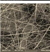
Clean Air NW 60 - textile filter media provides filtration of any dust particles, mold or fungal spores size greater than 2.5  $\mu$ m with 99,99 % efficiency. For its functioning is not necessary ventilation system with forced ventilation. This material is manufactured with using the most modern textile technologies takes advantage of the unique barrier quality of submicron fibers (nanofibers). By using nanofibrous structure material is highly permeable to air.
