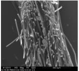
The material prevents the penetration of dust and pollutants from the air from the external environment into the interior. Filtration efficiency class F7 according EN 779.
